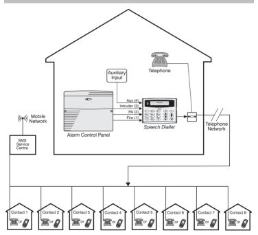
The Speech Dialler provides a means of communicating alarm information from an alarm control panel to a standard or mobile telephone. The unit is normally connected to an alarm control panel, which provides the necessary power and battery backup. The unit is also connected to a standard telephone line and behaves like another extension to the telephone and does not affect its normal operation or that of any other extension fitted.
